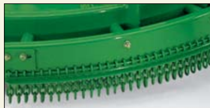
Front and rear safety chain shields are standard equipment on all John Deere CX, HX, and MX Series Rotary Cutters.
