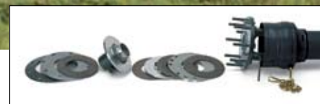
A self-adjusting four-plate slip-clutch helps protect the drivelines. The spring compression system is easily unloaded with six screws. This ensures that clutches are not sticking after extended periods of storage.
