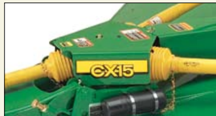
Driveshafts are encased in a protective sleeve which is chained in place. Don't leave the tractor before the PTO comes to a complete stop as blades can continue to rotate.
