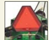
Slow Moving Vehicle (SMV) signs should be used when transporting and mowing along roadsides.
