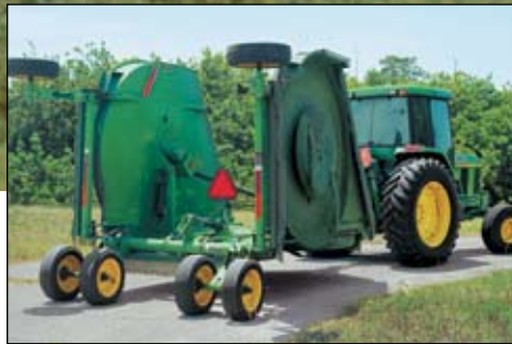
Wings flex from 90 degrees above (transport mode) to 22 degrees below grade. And the wings operate simultaneously for quick transition to and from transport mode with standard hydraulic lift and fold.
