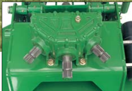
John Deere-built gearcases are backed by a 3-year warranty. Oil-level dipsticks with pressure checkvalves are found on each gearcase.
