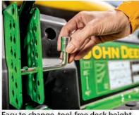
Easy to change, tool-free deck height adjustments in 1/4" increments.
