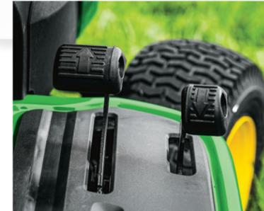
Two-pedal hydrostatic transmissions make maneuverability smooth & simple.
