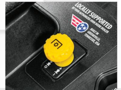
Electronic mower deck engagements increase efficiency with the pull of a button.
