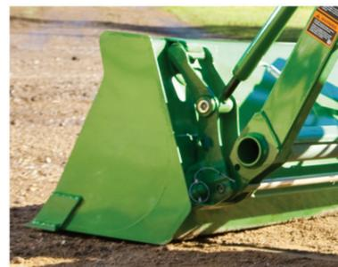
Change or remove a front loader attachment *without* tools in seconds.
