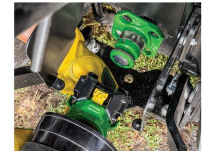
Quik Knect™ PTO receivers make for easy PTO connections in seconds.
