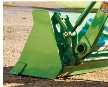
Change or remove a front loader attachment *without* tools in seconds.
